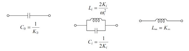
If Z(s) has no pole at the origin then capacitor  $C_0$  is not present in the network. Similarly, if there is no pole at  $\infty$ , inductor  $L_{\infty}$  is not present in the network.
