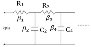
If Z(s) represents an admittance function, then the first Cauer form represents RL admittance realization. The admittance function in partial fraction is given by
